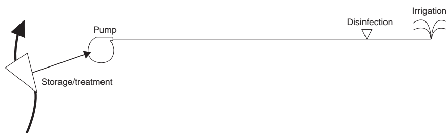
Figure 6.1 (b) Schematic of an example harvesting scheme with on-line storage
